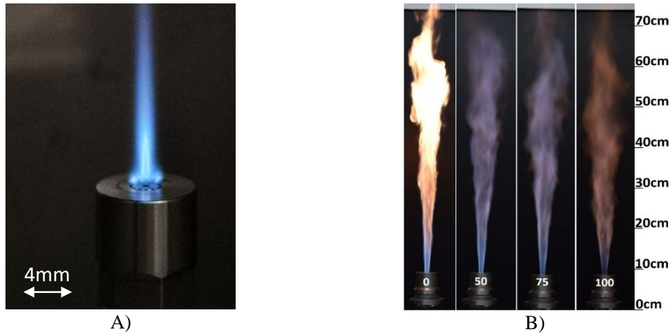
Figure 2. A) picture of a 1.2 kW premixed natural gas/oxygen flame and B) 35 kW oxyfuel-flames from 0 to 100 vol.% hydrogen admixture
